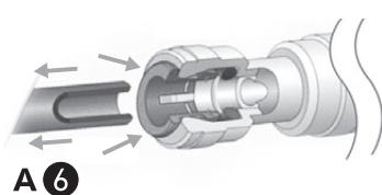
To disconnect the hose from the quick release fastener, the tap water supply hose (A-6) must not be under pressure. Remove the safety clip (A-11), push the safety ring all the way back and then pull the tap water supply hose (A-6) out of the quick release opening.
