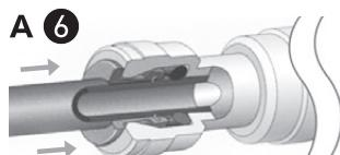
The tap water supply hose (A-6) must be inserted at least 1 cm into the quick release opening.
