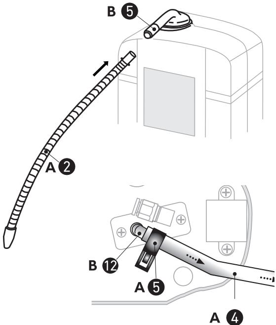
1. Screw the alkaline outlet hose (A-2) to the upper water outlet (B-5).
