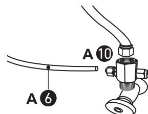
**CAUTION:** When assembling please make sure the connection pins on the T-piece do not bend sideways. This may cause a micro crack, which can even lead to breakage due to the constant water pressure.
