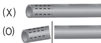
Always make sure that the tap water supply hose (A-6) is not bent or damaged in any way at the point of insertion into the quick release fastener opening. If this is the case, cut off the damaged piece.
