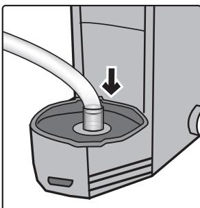
5. Connect the descaling pump to the power supply. The pump starts automatically.
