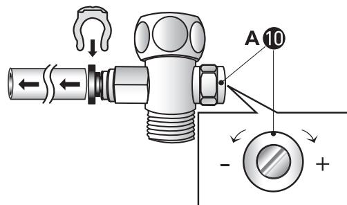
**Note:** If the water pressure is too high, the message "Error 4" or "Error F" appears on the display (B-22). If the water pressure is too low, the device switches off automatically.
