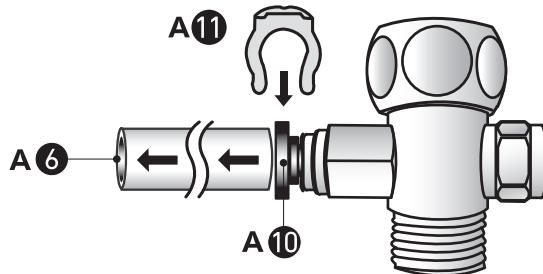
3. Pass the tap water supply hose (A-6) through an opening in the counter or sink (diameter at least 6 mm) to the position where you have placed the ECAIA ionizer S.
