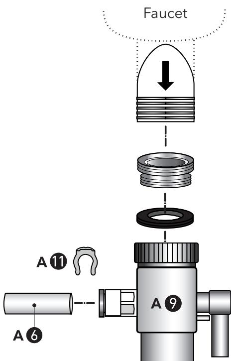
1. Remove the aerator from the faucet and replace it with the diverter valve (A-9). The intermediate thread is used depending on the type of a thread (internal or external thread).
