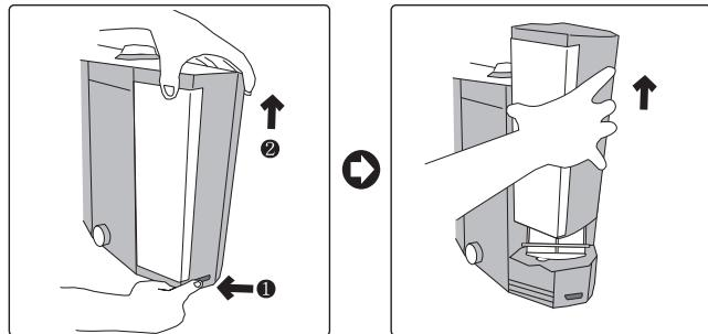
2. Disconnect the plug lock on the filter cable.
