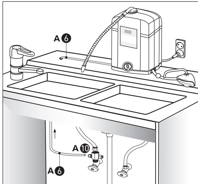
4. Connect the other end of the tap water supply hose (A-6) to the quick release fastener opening of the water inlet (B-11) on the bottom of the ECAIA ionizer S and fix the safety clip 1/4 " (A-11).
